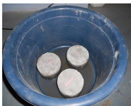
Figure.9. Sorptivity Test on M-sand Specimen
